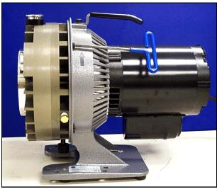
3. Remove the four M6x16 screws attaching pump module to the frame.
