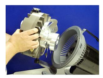
4. Remove pump module from the frame.
