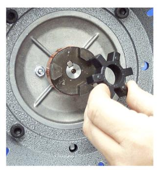
4. Insert spider in motor coupling.
