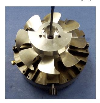
1. Install key in slot on crankshaft.
