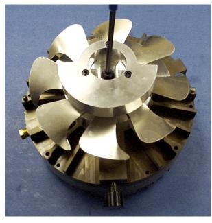
5. Remove M8x12 screw and washer attaching fan assembly to crankshaft.
